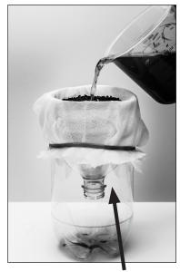
3. Water flows through filter material into the bottom of the bottle.
