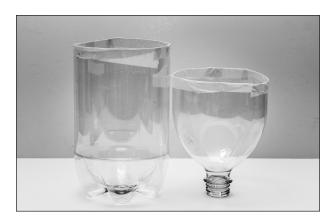
5. Stack top of bottle upside-down inside bottom of bottle. This is the Filter Base.
