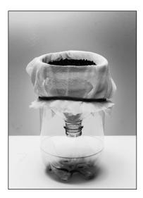
2. Pour a dirty water sample into the open top of the Filter Base.
