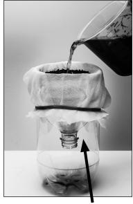
3. Water flows through the filter material into the bottom of the bottle.
