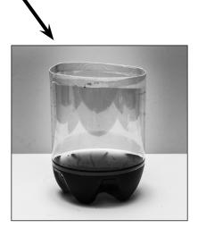
6. Repeat with each filter material by pouring a new sample of dirty water through each filter material.
