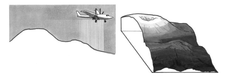
When all of those distances are placed together, they create a 3D image, similar to the way the pins on a pinscreen toy show the shape of the object underneath it.
