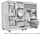
This water filtration system uses complex processes to remove salt and body waste from water in space.
