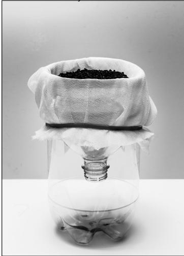
2. Pour dirty water sample into open top of the Filter Base.
