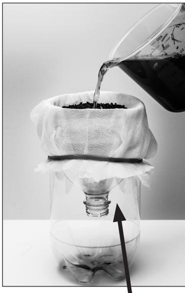
3. Water flows through filter material into the bottom of the bottle.
