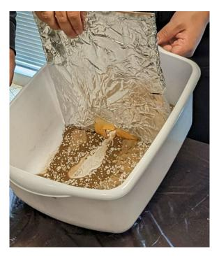
3. A close-up view of the alluvial fan barrier. The one-inch notch allows water to flow through and create a fan-like shape in the sand. This barrier simulates what happens to water when it flows from a mountainous area where it can't spread out, into a low-lying flat area where it can spread out. Science Activity 1 Image of Mars
